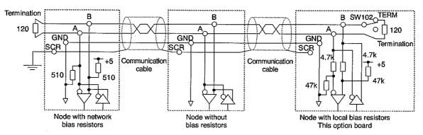
N.B.:Do not connect the SCR terminal to the power ground of inverters or other units.
